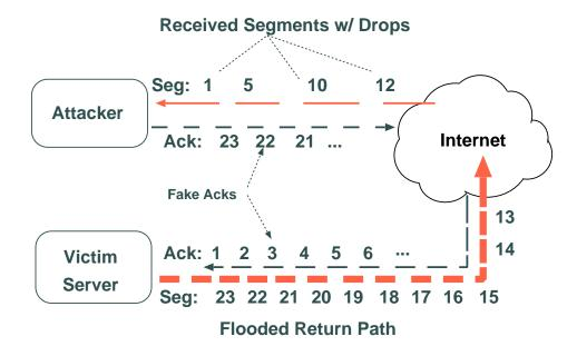
Attack network core by causing well-provisioned servers to send lots of traffic (GBs) into the core by sending fake TCP ACKs
